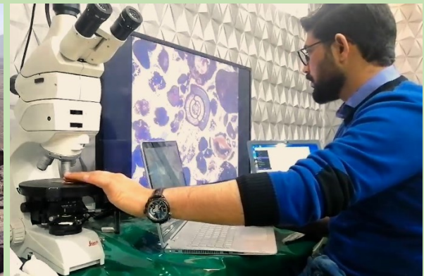
A GSP geologist performing petrographic analyses, as part of an R&D project, to determine the mineral content of the rocks.
