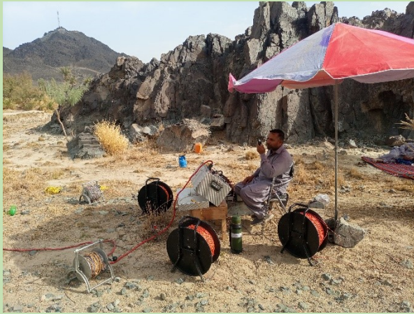
A Geophysicist performing Induced Polarization (IP) Survey for the exploration of Sulphide Mineralization (i.e., Copper) in Chagai, Balochistan, as part of R&D project.
