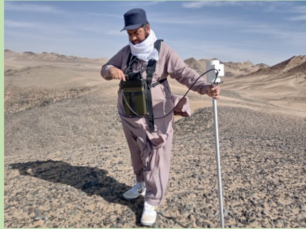
A Geophysicist performing Magnetic Survey for the ground follow up of aeromagnetic anomalies in Nokkundi, District Chagai, Balochistan.
