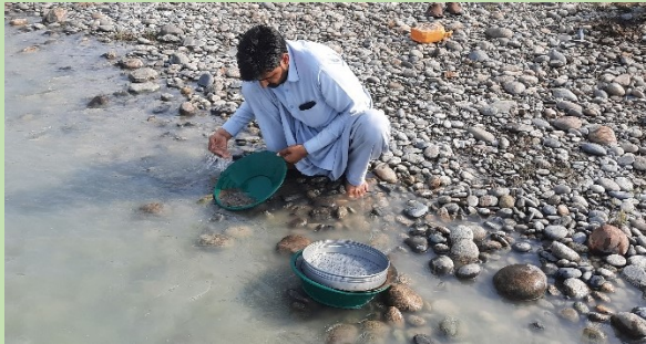
A geologist performing panning as part of the Placer Project to explore gold and other heavy minerals along the Indus River in District Attock, Punjab.
