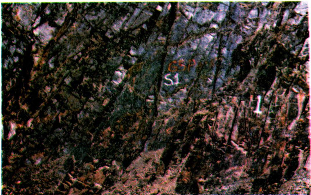
PLATE - 2 Jointing pattern in the phyllite rocks causing small fragmentation of the formation.
